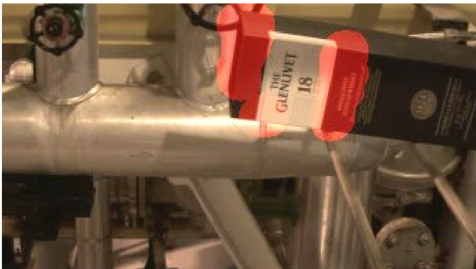
Figure 4.14: Result with the introduction of the second codebook when the abandoned object is a whisky box. The detected area is smaller, but the false detections disappear.
