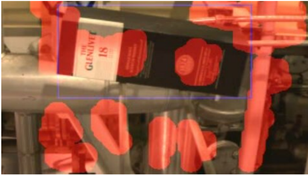
Figure 3.12: Example of results obtained with a moving camera when the abandoned object was a whisky box. In most of the frames, it was not possible to find a threshold where only the abandoned object was detected.
