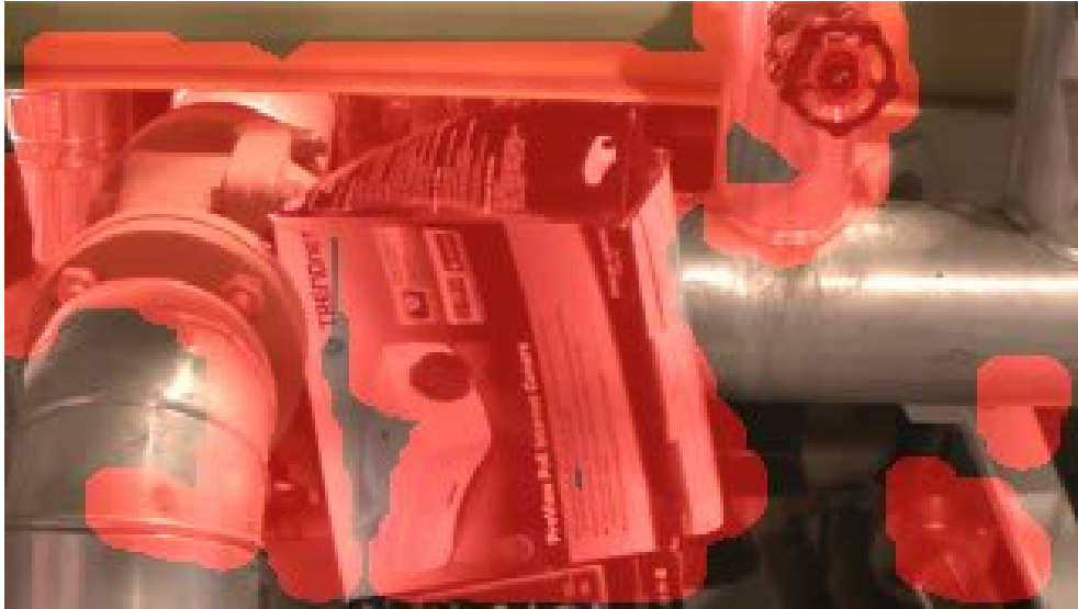
Figure 4.17: Result with only the first codebook when the abandoned object is a camera box. There are several false detections.
