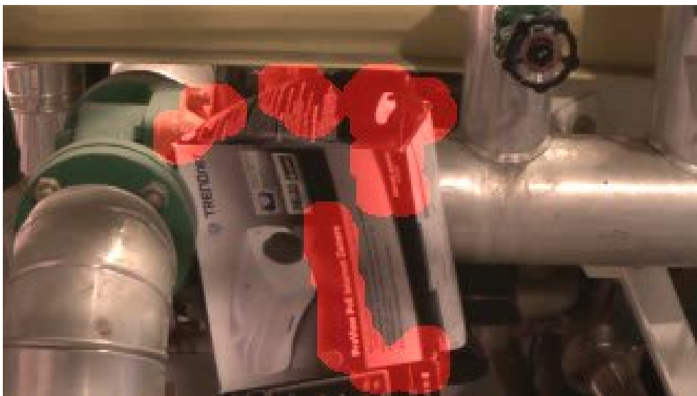
Figure 4.18: Result with the introduction of the second codebook when the abandoned object is a camera box. The detected area is smaller, but the false detections disappear.
